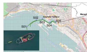
Fig. 3. Glider track in Saumaty Harbor near Marseille city (glider towed behind a small boat). Surface water was sampled at S01-S05 wps for naphthalene and phenanthrene laboratory GC/MS analysis. Photo credit: Jay Pearlman.
